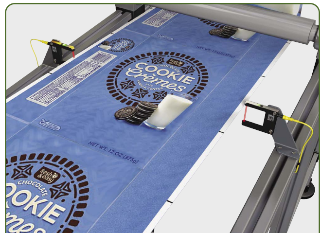
Web alignment application – Two 45LSP fork sensors monitor horizontal film position on both sides of the roll. If the film drifts in either direction the sensor's light beam will be interrupted, causing the machine's dancer arm to correct the film position.
