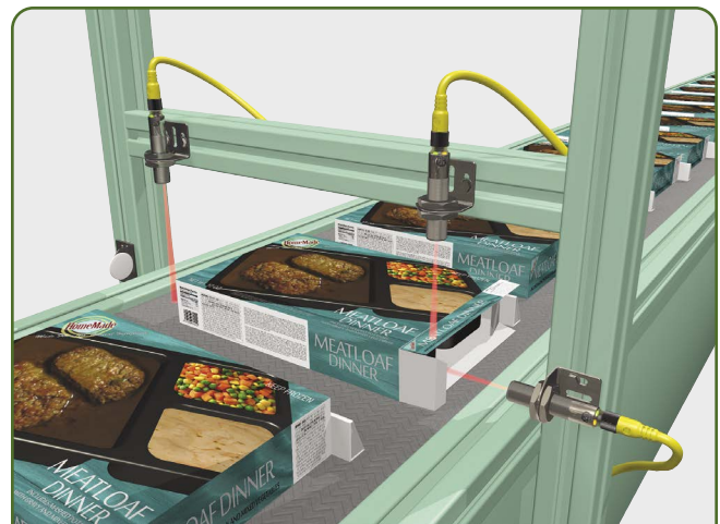
Flap detection - When the single 42CS mounted on the side of the conveyor senses a food package, it triggers the two sensors above to check for open box flaps, ensuring all packages are sealed.
